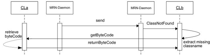
**Fig. 5** Sequence diagram for point-to-point code mobility
