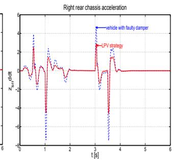
Fig. 17. Chassis acceleration in rear right  $\ddot{z}_{s_{rr}}$ .
