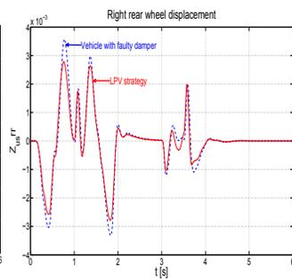
Fig. 9. Wheel displacement in rear right  $z_{us_{rr}}$ .
