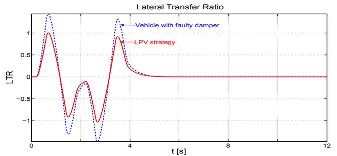
Fig. 3. Lateral load transfer
