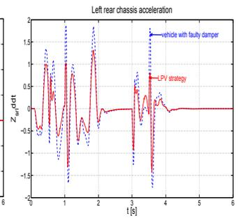
Fig. 19. Chassis acceleration in rear left  $\ddot{z}_{s_{rl}}$ .
