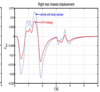
Fig. 13. Chassis displacement in rear right  $z_{s_{rr}}$ .
