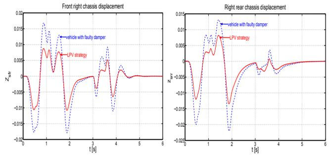
Fig. 12. Chassis displacement in front right  $z_{s_{fr}}$ .
