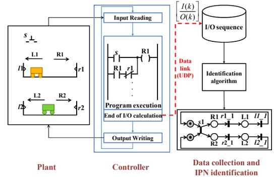
Fig. 1.  $\{\text{PLC} + \text{Plant}\}$  compound and identification procedure.
