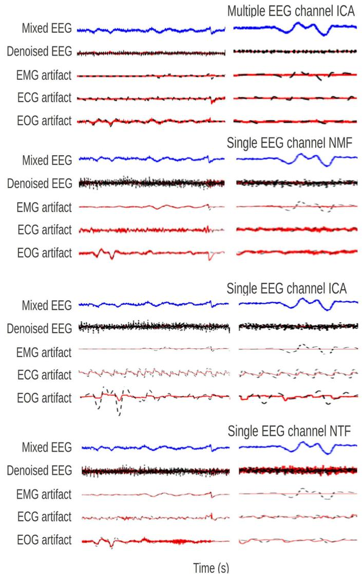
**Fig. 2.** Signal decomposition on two pieces of a single EEG channel recordings located in the temporal brain area for each separation source method. In order of appearance, the blue signal is the original signal, the red signal is the denoised signal and the last three signals respectively include the EMG, ECG and EOG signal in black dotted line and the estimated artifact signal in red solid line.
