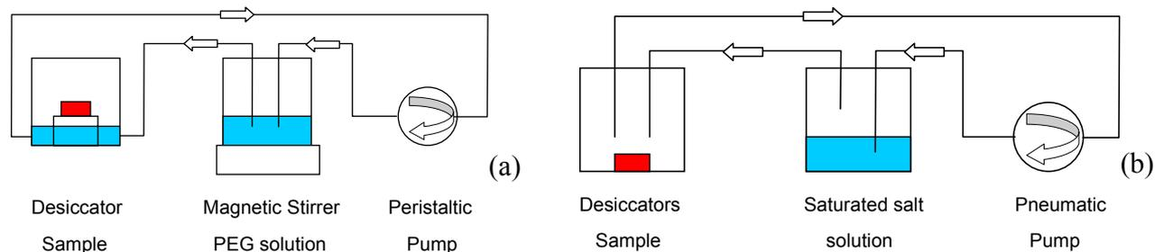
Figure 3. Vapour phase control: (a) using PEG solution, (b) using saturated salt solutions.
