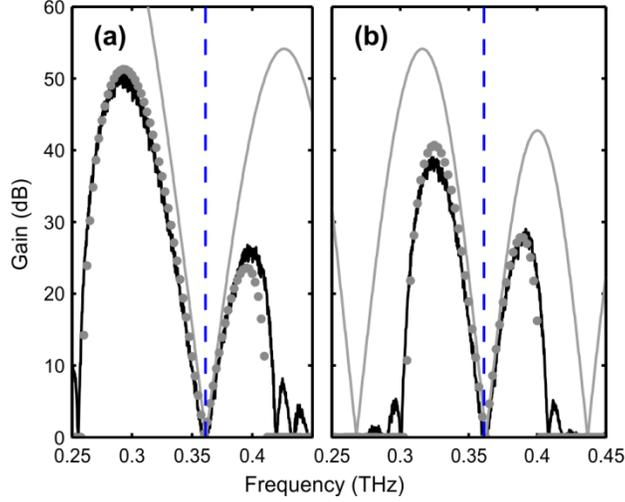
**Figure 6 :** Output spectrum after 12 kilometers of propagation obtained from numerical simulations (black line), from analytical equation (grey line) and from the Floquet linear stability analysis (grey circles): (a)  $D_{amp} = 3.7$  ps/km/nm; (b)  $D_{amp} = 6.7$  ps/km/nm.
