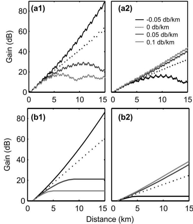
**Figure 10 :** Longitudinal evolution of the gain for the inner and outer sub-sidebands (panels (a1,b1) and (a2,b2) respectively) for different levels of attenuations/losses: -0.05, 0, 0.05 and 0.1 dB/km, solid black, dotted black, dark grey and light grey lines respectively. Results from numerical simulations (a1,a2) are compared with the results predicted by Eq. 9 (b1,b2).
