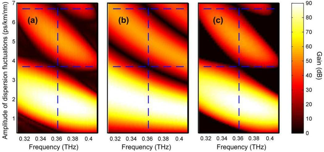
**Figure 5 :** Magnification of the MI gain spectrum around the first QPM sideband vs.  $D_{amp}$ . Numerical results (a) are compared with the analytical results (b) predicted by Eq. (8) and by the Floquet linear stability analysis (c). Blue dashed vertical lines indicates the angular frequency  $\Omega_l$  as predicted from Eq. (0) and horizontal lines highlight the values of dispersion fluctuations that are then used in Fig. 6.
