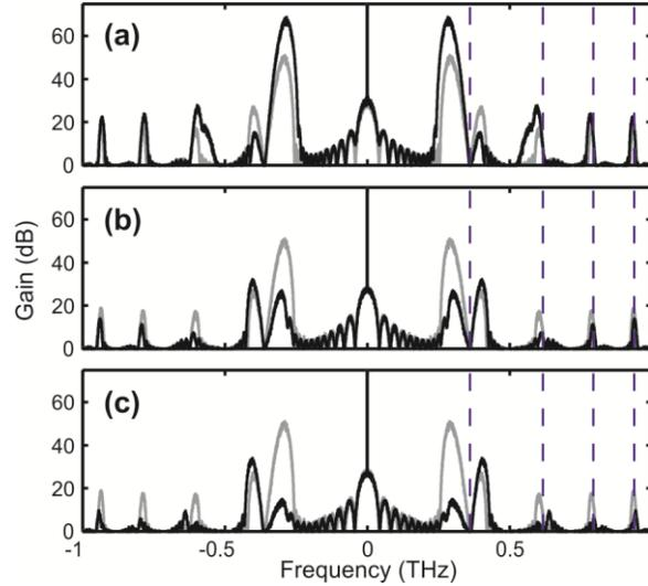
**Figure 7 :** Evolution of the output spectra after 12 kilometers of propagation for different levels of losses or gain (solid black lines): (a) 0.05 dB/km of gain. (b) 0.05 dB/km of loss. (c) 0.1 dB/km of loss. Results obtained without losses are plotted with grey solid lines.
