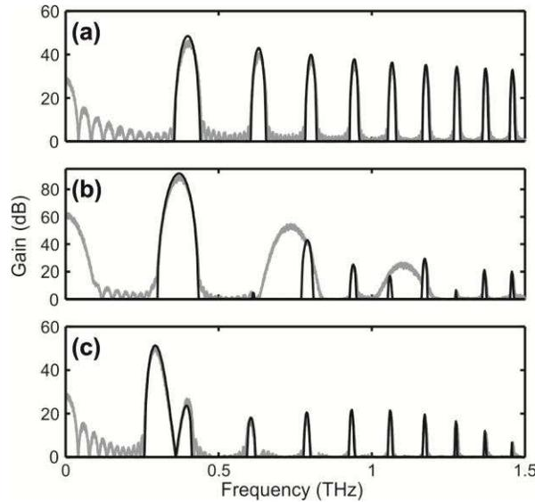
**Figure 2 :** Anti-Stokes sideband spectrum as Fig.1. The results from the Floquet linear stability analysis of the NLSE with periodic dispersion (black lines) are compared with the results of the numerical integration of Eq. (1) (grey lines)
