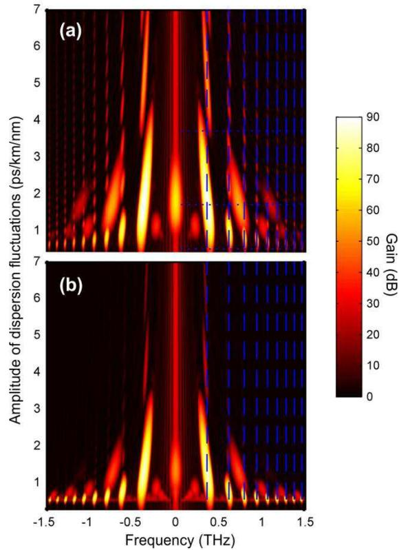
**Figure 3 :** Evolution of the output MI spectrum after a distance of 12 kilometers according to the level of dispersion fluctuations. (a) Results obtained for a sinusoidal dispersion modulation. (b) Results obtained for a square dispersion modulation. The position of the sidebands predicted from Eq. (0) is plotted with vertical dashed lines. The spectra corresponding to cases of Fig. 1 are highlighted by dashed horizontal lines.
