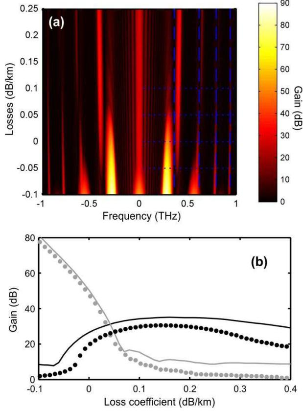
**Figure 8 :** (a) Evolution of the output spectrum after 12 kilometers of propagation according to the level of linear losses/gain. (b) Evolution of the parametric gain experienced by inner and outer sidebands (grey and black lines or symbols, respectively) according to the level of linear losses/gain. The numerical results (solid lines) are compared with results based on Eq. 9 (dots).
