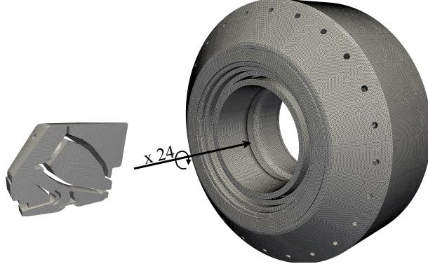
Figure 5: Mesh used for the discretization of an industrial gas turbine combustor. The number of nodes is  $n = 1,782,384$ .
