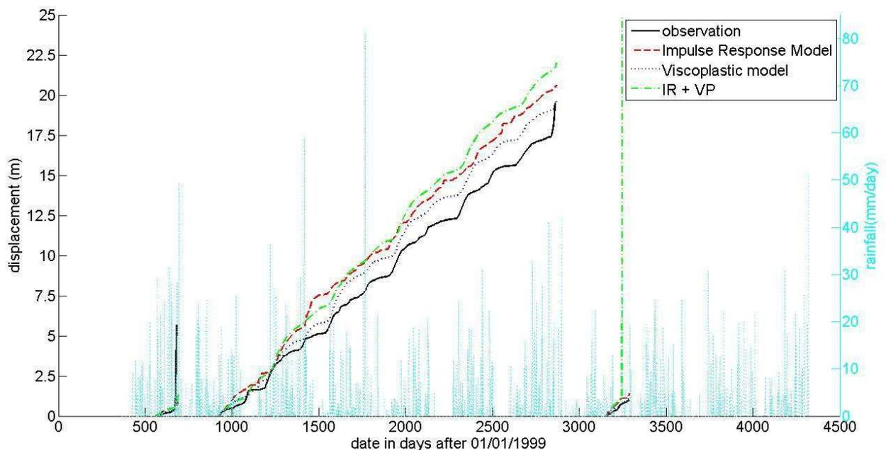
Figure 4 – Predicted and observed cumulated displacements
