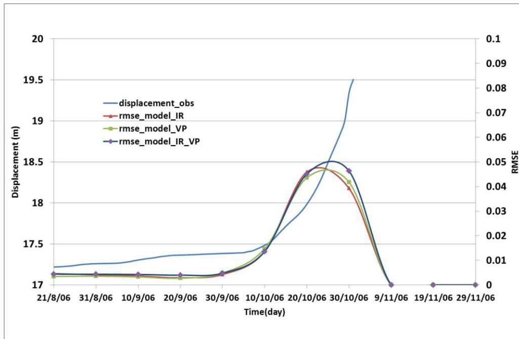
Figure 5 – Observed displacement and RMSE computed before the flow
