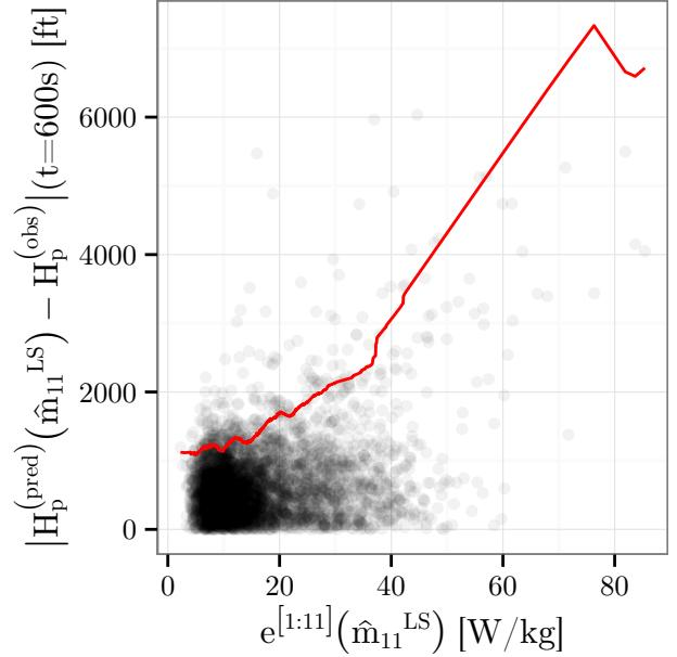
Figure 3: Relation between  $e^{[1:11]}(\hat{m}_{11}^{LS})$  and the absolute error on the predicted altitude  $|H_p^{(pred)}(\hat{m}_{11}^{LS}) - H_p^{(obs)}|(t = 600\text{ s})$ . The red line is the estimated 95 % quantile. It is obtained by local linear quantile regression [28].
