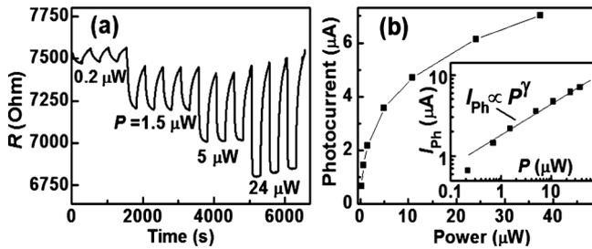
FIG. 2. (a) Modulation of the resistance of the EO-EG channel under square-wave pulses of blue LED illumination of different power. (b) Dependence of EO-EG channel photocurrent  $I_{\text{Ph}}$  on the power  $P$  of incident radiation. Inset shows the same dependence in double-logarithmic scales.
