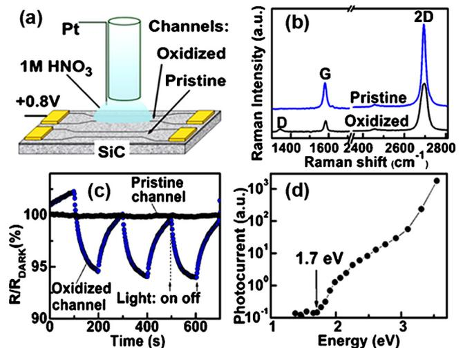
FIG. 1. (Color online) (a) Schematic of electro-oxidation experiment; (b) Raman spectra of pristine and EO-EG ( $\lambda_{\text{laser}} = 532$  nm); (c) effect of fluorescent room light illumination on the resistance of EO and pristine EG channels. (d) Spectral dependence of photoresponse of the EO channel.
