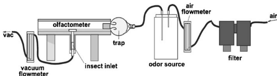
**Figure 1.** Lateral view of the four-way olfactometer (modified from Carroll et al., in preparation). The olfactometer is connected to an insect inlet port attached to the vacuum, drawing air from the odor source over the insect as it is released into the olfactometer. The vacuum is attached to a flowmeter (2 l/min) drawing four times the air delivered by each of the four ports (0.5 l/min), each port delivering air through air flowmeters, odor sources, and glass traps.
