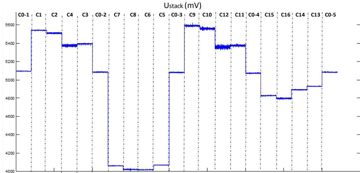
Figure 4-10 Stationary signals of the stack voltage in 20 tests (from VTT 1<sup>st</sup> test round data)
