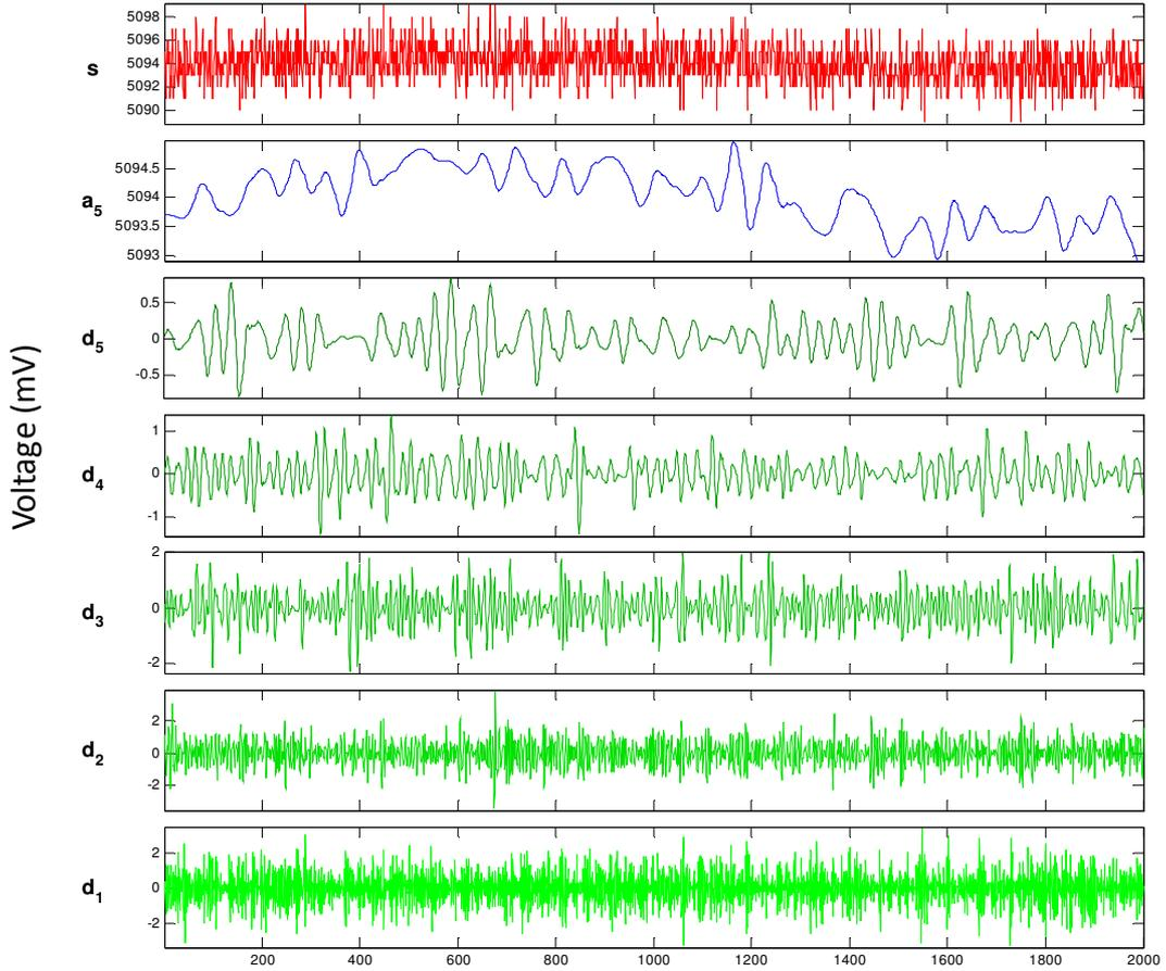
Figure 4-7 An example to show the results of a 5-level discrete WT on an SOFC's voltage signal (the original signal: **S**)
