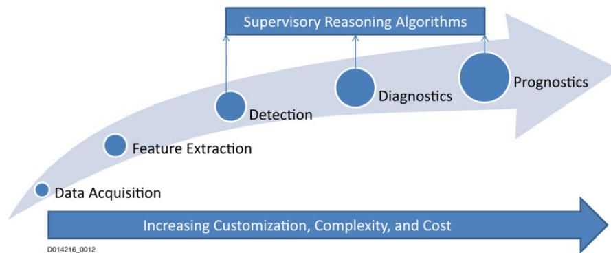
Figure 2-2 The complete process of condition-based maintenance [SRI'09]
