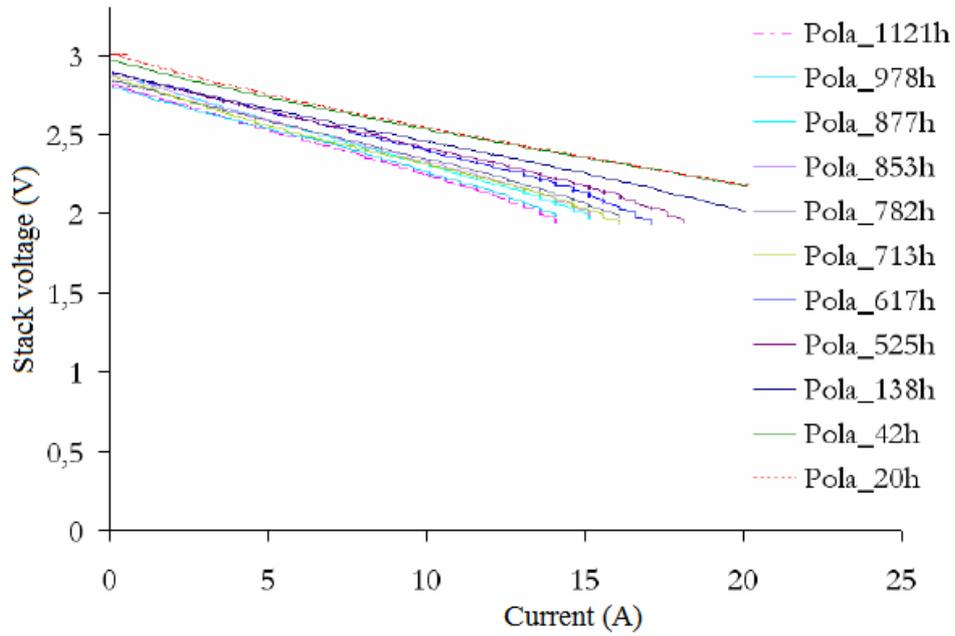
Figure 4-26 Polarization curves of the SOFC stack
