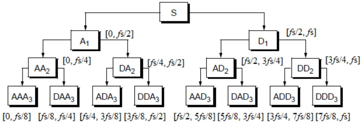
Figure 4-4 Wavelet packet decomposition tree for a digital signal sampled in frequency  $f_s$  [Misiti'09]
