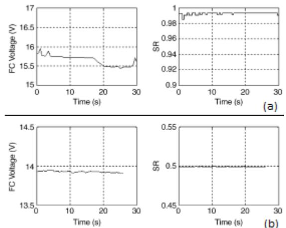
Figure 2-11 Evolution of voltage and SR for different operating temperatures. (a) At 18°C; (b) at 50°C (drying) [Hissel'04]
