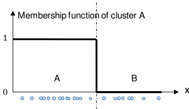
Figure 3-2 Classification by  $k$ -means method
