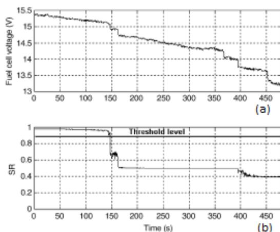
Figure 2-10 Evolution of voltage and SR when the flooding phenomenon occurs; (a) FC voltage and (b) SR value [Hissel'04].
