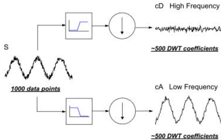
Figure 4-2 Schematic diagram of one-stage filtering [Misiti'09]
