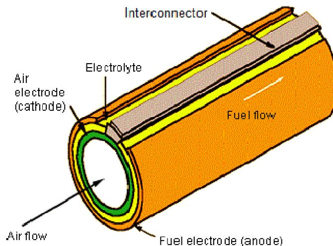
Figure 1-3 Siemens-Westinghouse single tubular SOFC\*
