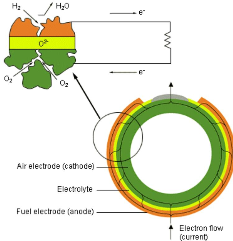
Figure 1-4 Single tubular SOFC operation and current path\*
