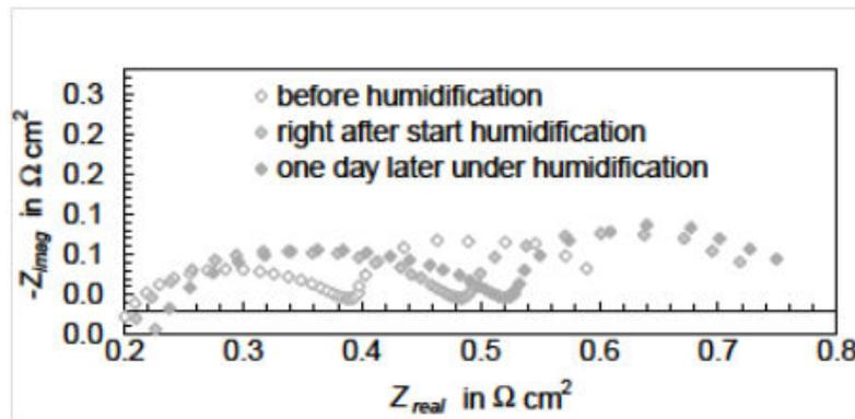
Figure 1-6 Impedance spectra recorded under current density at  $750^\circ\text{C}$  and  $0.75\text{A}/\text{cm}^2$  just before starting the 4% humidification of air, right after start and after one day in humid air [Hagen'09].
