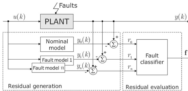
Figure 2-3 Schema of process model-based fault diagnosis [Isermann'06]
