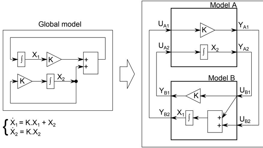
Figure 2: Loop creation due to the model splitting
