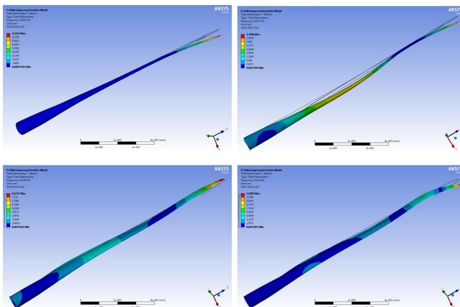
Figure 5: Four natural vibration modes of the rotor blade on two supports according to Figure 2 (simulation)
