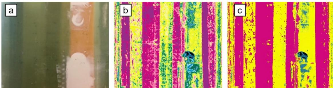
Figure 7: Results of ultrasonic scan on a rotor blade section; a) photo of the test section, b) ultrasonic scan with 64 colours, c) ultrasonic scan with only 5 colour grades giving a better position of manufacturing defects (e.g. voids in glue are red points in a yellow band)
