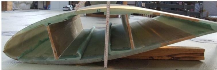
Figure 6: Cross-section of a rotor blade segment with manufacturing faults
