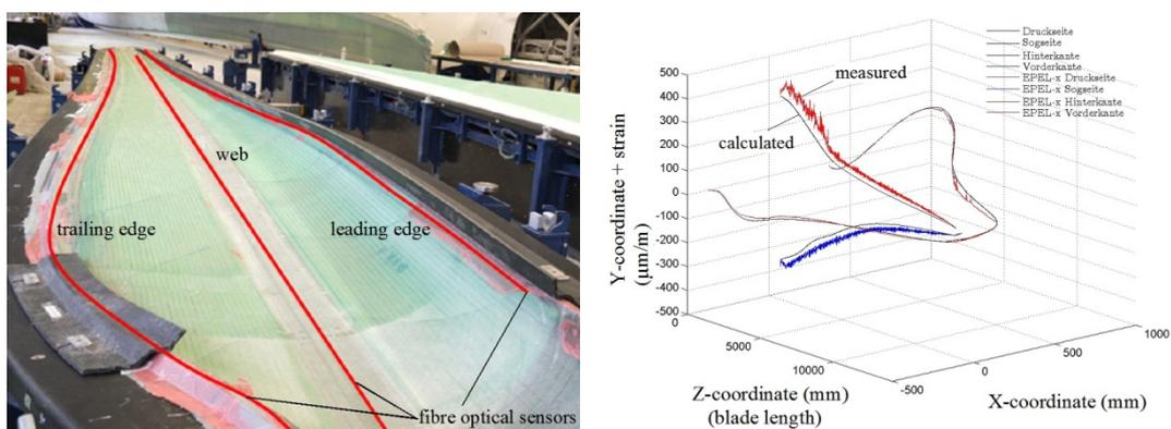
Figure 4: Locations of the fibre optical sensors in the rotor blade (left) and comparison of measured and simulated strains along the fibers (right)
