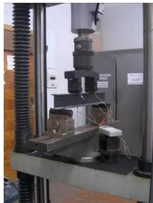
Figure 4. Four point bending experimental system
