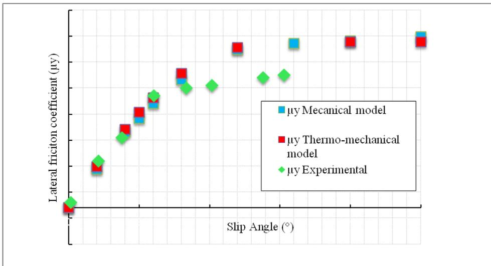
Fig. 7. Comparison between experimental data, mechanical and thermo-mechanical models
