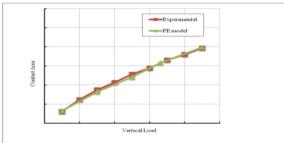
Fig.4. Evolution of contact area in the case of a grooved tire
