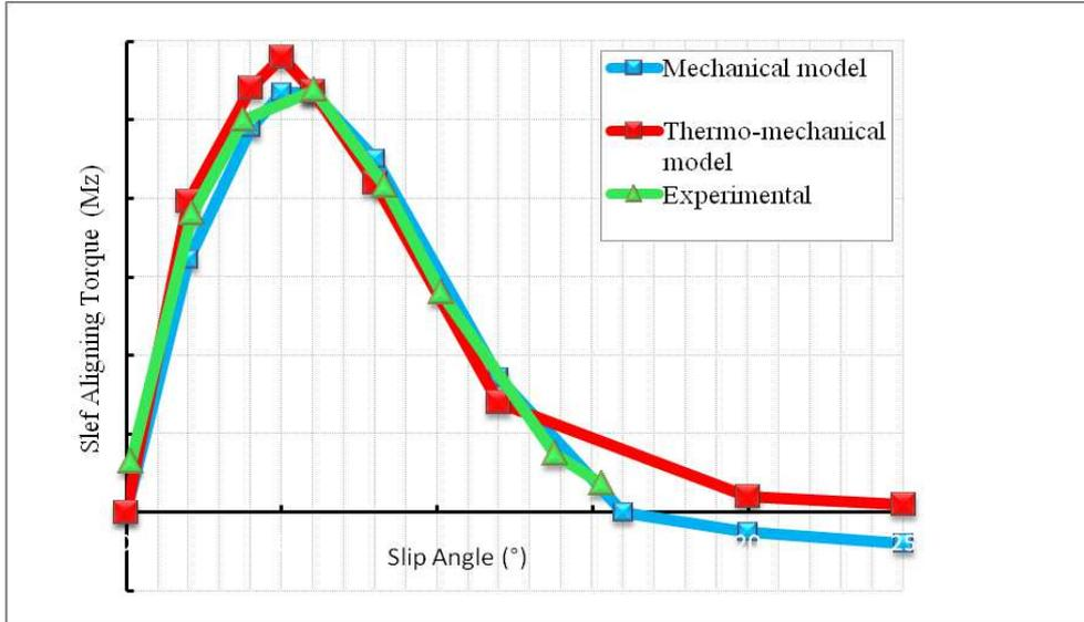
Fig. 6. Comparison between experimental data, mechanical and thermo-mechanical models
