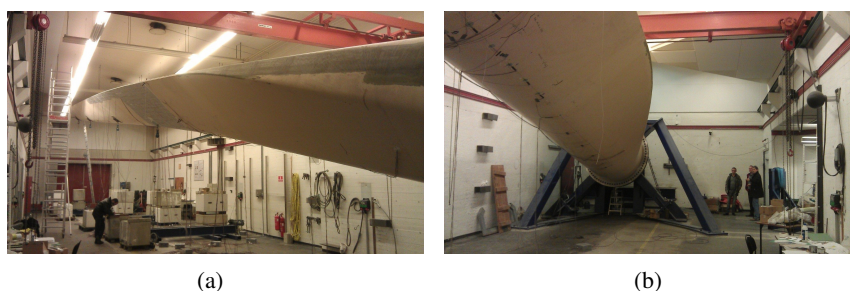
Figure 1 : SSP 34 m blade mounted on the test rig. (a) Root-to-tip view. (b) Tip-to-root view.
