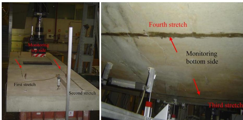
Figure 2: Load arrangement and location of optical fiber and joint opening sensors
