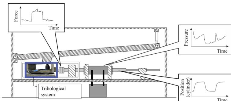
Figure 1: Wear test rig, Chair of Dynamics and Control, U Duisburg-Essen, Germany
