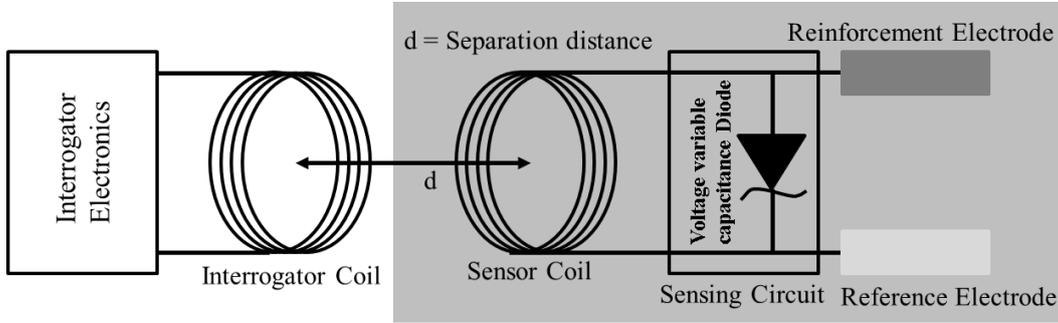
Figure 1: Block diagram of coupled coil sensor
