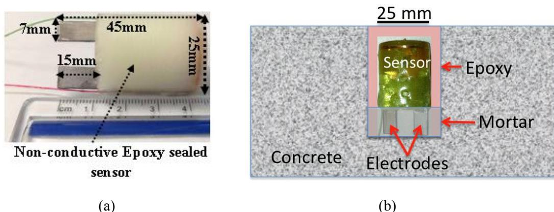
Figure 7: (a) Sealed sensor which is ready to be embedded (b) Sensor is  $\sim$ 25mm in diameter and is intended to be embedded into mortar placed in the bottom of a hole drilled into the concrete. Chlorides diffuse into the mortar leading to a rise in the corrosion potential. The potential can be measured using external coils. The potential can be read with 10 mV resolution.
