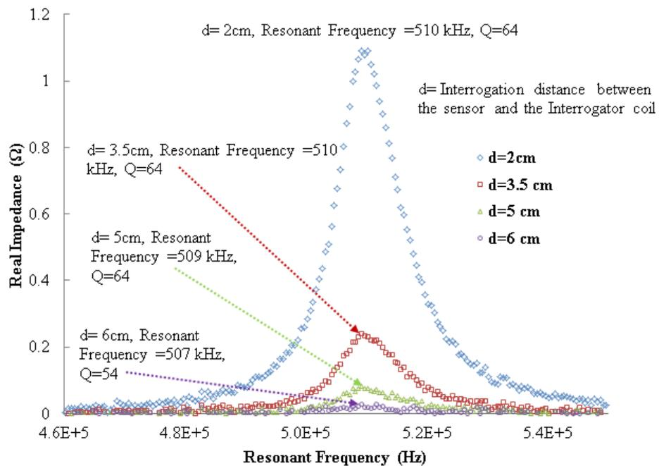
Figure 5: Sensor performance with separation distance
