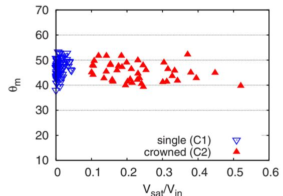
FIG. 7. (Color online) Measured opening angles  $\theta_m$  of single and crowned cap bubbles plotted vs the ratio  $V_{sat}/V_{in}$ . The data used to generate this figure are available online as supplemental material (Ref. 14).
