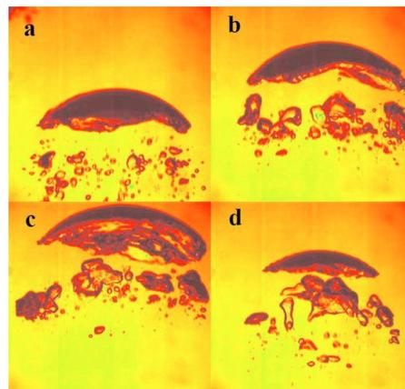
FIG. 3. (Color online) Pictures of typical crowned cap bubbles with, respectively, (a)  $V_{\text{in}}=114 \text{ cm}^3$ ,  $V_{\text{sat}}/V_{\text{in}}=0.05$ ; (b)  $V_{\text{in}}=126 \text{ cm}^3$ ,  $V_{\text{sat}}/V_{\text{in}}=0.15$ ; (c)  $V_{\text{in}}=144 \text{ cm}^3$ ,  $V_{\text{sat}}/V_{\text{in}}=0.3$ ; and (d)  $V_{\text{in}}=66 \text{ cm}^3$ ,  $V_{\text{sat}}/V_{\text{in}}=0.5$ .
