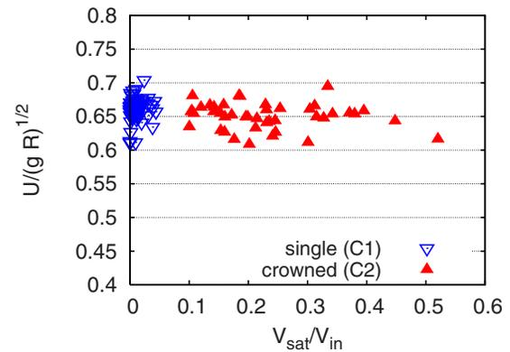
FIG. 6. (Color online) Measured individual Davies and Taylor ratios  $U/\sqrt{gR}$  of single and crowned cap bubbles plotted vs the ratio of the estimated volume  $V_{sat}$  contained in the satellite bubbles to the total injected volume of gas  $V_{in}$ . The ratio predicted by the theory of Davies and Taylor (Ref. 11) is  $2/3 = 0.6666$ . The data used to generate this figure are available online as supplemental material (Ref. 14).
