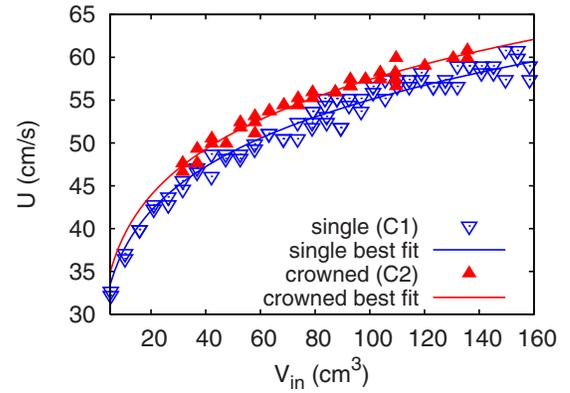
FIG. 4. (Color online) Rise speed  $U$  vs total injected volume of air for single cap bubbles ( $V_{sat}/V_{in} < 0.05$ ) generated with the C1 cup and crowned cap bubbles ( $V_{sat}/V_{in} > 0.1$ ) generated with the C2 cup. The best-fit curves have been computed by assuming  $U = Fr g^{1/2} V_{in}^{1/6}$  and then computing the best-fit Froude number  $Fr$ . The data used to generate this figure are available online as supplemental material (Ref. 14).
