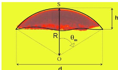
FIG. 2. (Color online) Geometry of a single spherical cap bubble. Picture of a single spherical cap bubble of air ( $V=68 \text{ cm}^3$ ) rising in still water at constant speed  $U$ .  $R$  is the radius of curvature of the bubble at the front stagnation point  $S$ , while  $\theta_m$  is its subtended half-angle;  $h$  and  $d$  are the height and width of the bubble, respectively.
