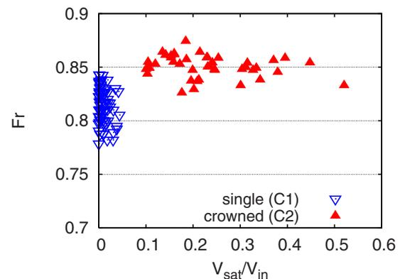
FIG. 5. (Color online) Measured individual Froude numbers of single and crowned cap bubbles plotted vs the ratio of the estimated volume  $V_{sat}$  contained in the satellite bubbles to the total injected volume of gas  $V_{in}$ . The data used to generate this figure are available online as supplemental material (Ref. 14).
