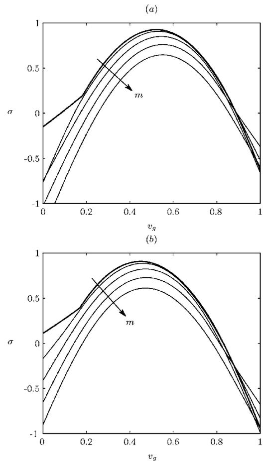
FIG. 4. Growth rates  $\sigma$  of the axisymmetric  $m=0$  mode (thick line) and azimuthal modes  $m=1, 2, 3, 4$  in a thin shear layer jet;  $R/\theta=20$ ,  $\text{Re}=\infty$ ,  $\text{Ma}=0$ . (a)  $S=1$ ; (b)  $S=0.5$ .
