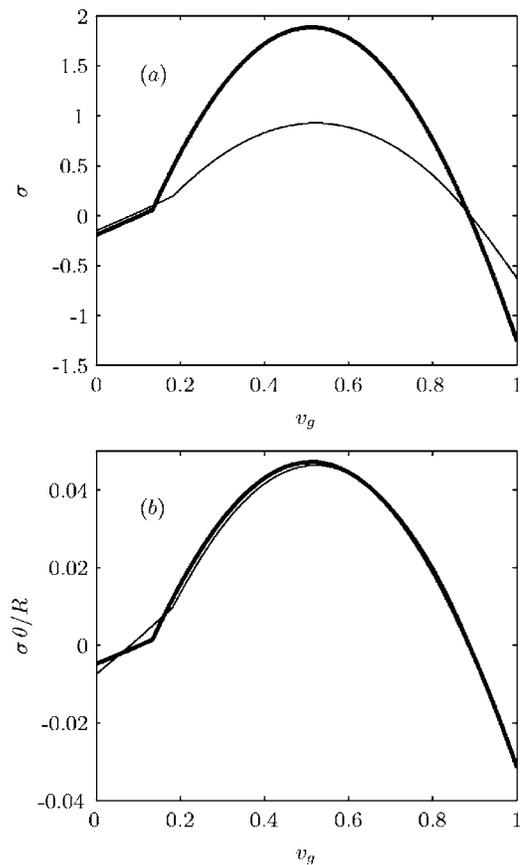
FIG. 2. Comparison of the spatiotemporal growth rates  $\sigma$  in jets for  $R/\theta = 20$  (thin line) and  $R/\theta = 40$  (thick line);  $m = 0$ ,  $S = 1$ ,  $\text{Re} = \infty$ ,  $\text{Ma} = 0$ . (a)  $\sigma$  scaled with jet radius  $R$ ; (b)  $\sigma$  scaled with shear layer thickness  $\theta$ .
