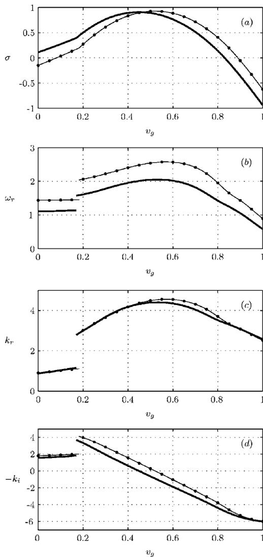
FIG. 1. Axisymmetric linear impulse response for flow parameters  $R/\theta = 20$ ,  $\text{Re} = \infty$ ,  $\text{Ma} = 0$ . Isothermal case  $S = 1$  (thin line); heated case  $S = 0.5$  (thick line); heated case  $S = 0.5$  in the absence of baroclinic torque ( $\bullet$ ). (a) Spatiotemporal growth rate; (b) real frequency; (c) real wave number; (d) spatial growth rate, all as functions of group velocity  $v_g$ .
