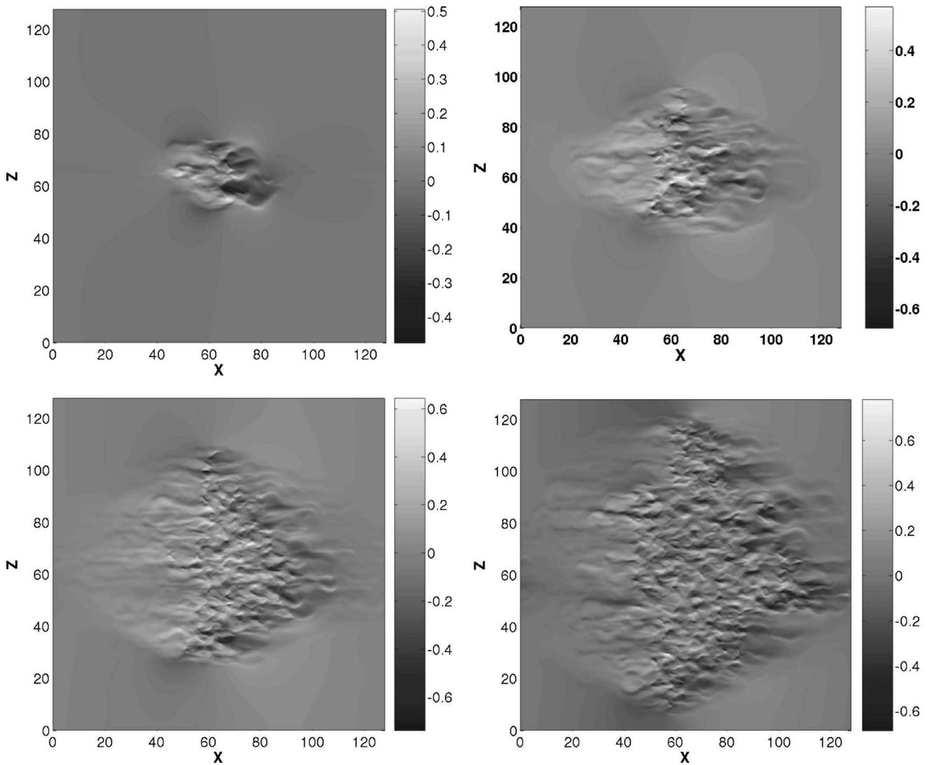
FIG. 1. Growth of a turbulent spot at  $R=250$  in a wide domain ( $L_x \times L_z = 128 \times 128$ ). Field of amplitude  $U_0(x, z, t)$  in gray levels at  $t=50, 150, 250$ , and  $350$  (from left to right and top to bottom). The whole domain becomes uniformly turbulent at  $t \approx 700$ .
