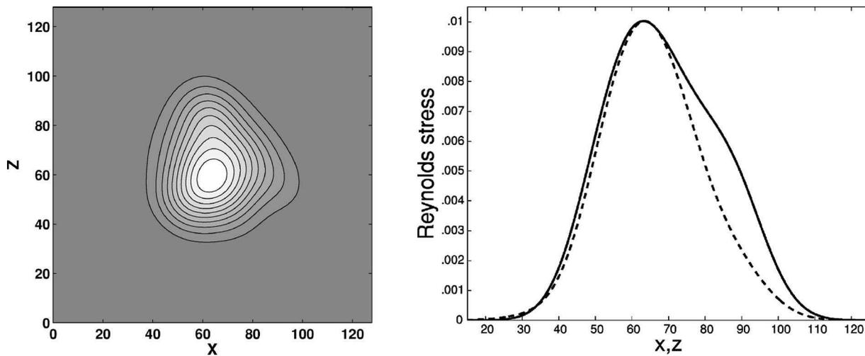
FIG. 6. Distribution of the averaged Reynolds stress field  $-\overline{U_0^s V_1^s}$  (left) and its variations along streamwise (solid line) and spanwise (dashed line) cuts through the maximum of the distribution taken as the center of the spot at  $x_c=64$ ,  $z_c=60$  (right).
