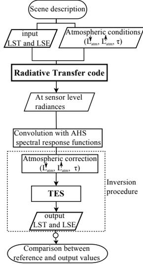
Fig. 1. Procedure overview, where  $L_{atm}^{\downarrow}$  is the downwelling atmospheric radiance,  $L_{atm}^{\uparrow}$  is the upwelling atmospheric radiance and  $\tau$  is the upwelling atmosphere transmission.
