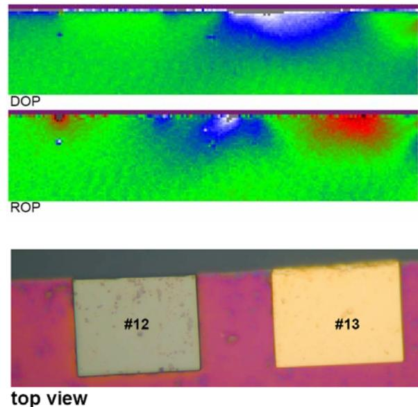
Fig. 6: Maps of the DOP and ROP over an area of  $180 \mu\text{m} \times 40 \mu\text{m}$  on the facet for a cleave through a pcm area. An image of the top of the pcm area is shown.
