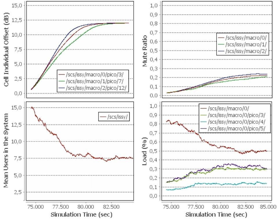
Fig. 7. Evolution of the KPIs and the key SON parameters, as visualized by the AutoSDN controller
