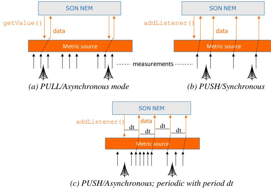
Fig. 2. The three supported modes of metric data exchange by AutoSDN
