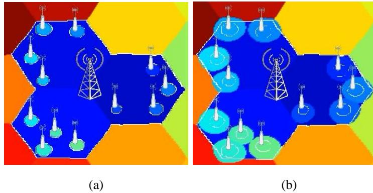
Fig. 6. (left) coverage map produced by the simulator with no SON functions; (right) increased CRE of the picos after activation of the LB SON
