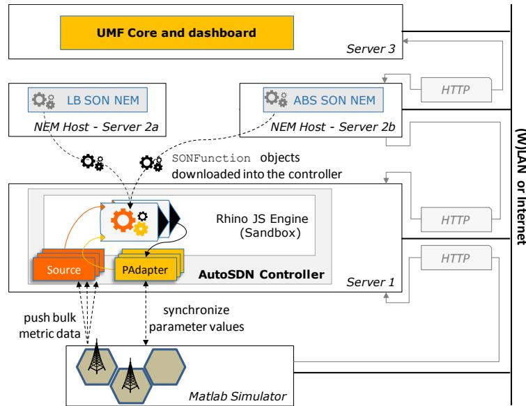
Fig. 4. System view of the AutoSDN prototype setup
