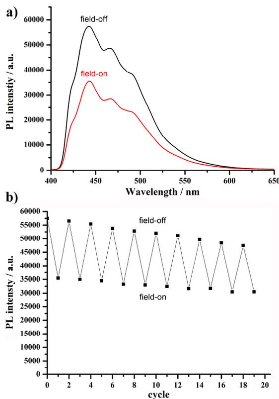
**Figure 10.** a) Emission spectra measured in field-off (0V) and field-on (20V); b) Time-dependent switching of PL intensity in response to several cycles of field-off (0V) and field-on (20V) ( $\lambda_{\text{ex}} = 340\text{-}380\text{ nm}$ ) ( $[\mathbf{1}] = 0.1\text{ \% w/w}$  in 5CB).
