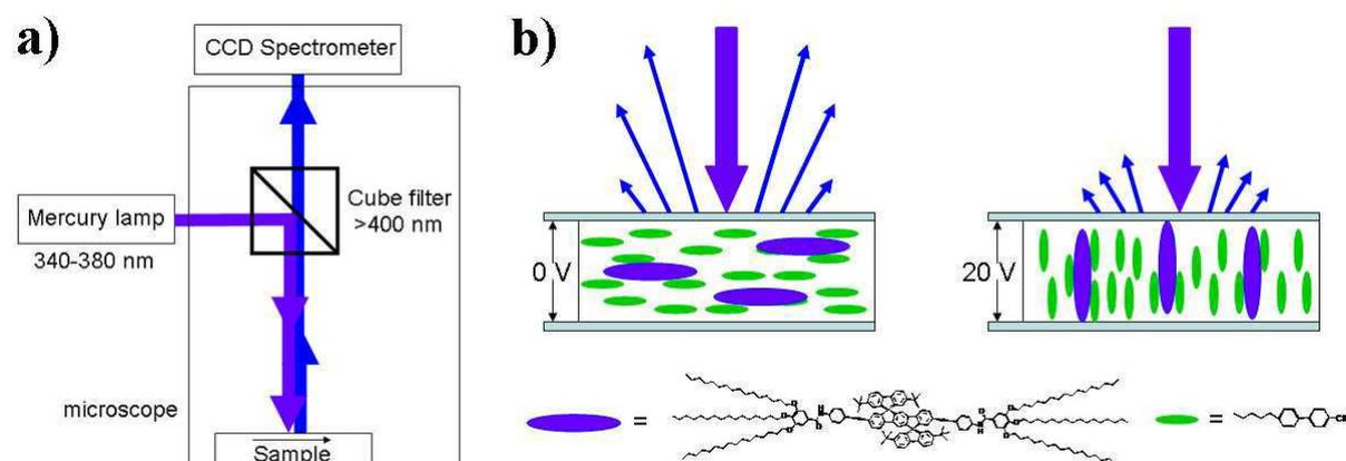
Figure 9. (a) Experimental setup for polarized photoluminescence measurements with compound **1**/5CB mixtures; (b) Schematic representation of the molecular organisation inside the LC cell without and with applied electric field and effect on the emitted blue light.
