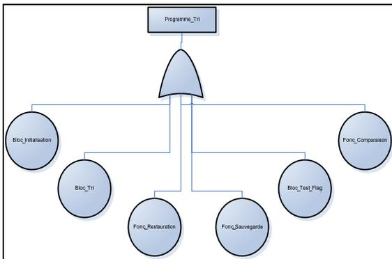
Fig.12. Fault tree of sorting program with tolerance.
