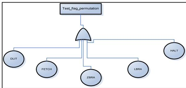
Fig.9. Fault tree of the Test\_Flag bloc
