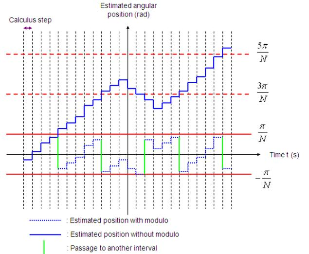
Fig. 2. Discontinuity point detection and position reconstruction algorithm
