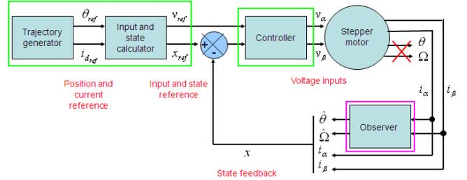
Fig. 1. Sensorless control scheme for the stepper motor
