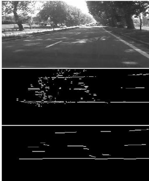
Figure 4 (top) the camera image; (middle) result of edge detection; (bottom) result of lane mark segment detection;
