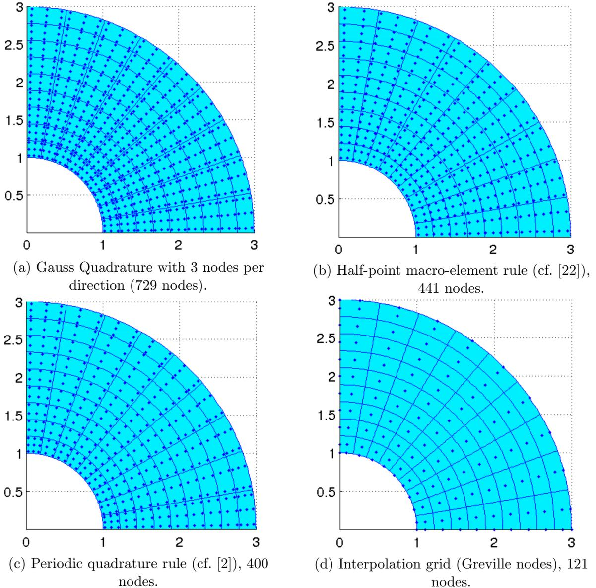
Fig. 2. Evaluation points for different numerical integration rules, for a  $9 \times 9$  quadratic B-spline discretization of a quarter annulus. The new approach uses the grid in (d), but has a higher cost per evaluation point than the other approaches.
