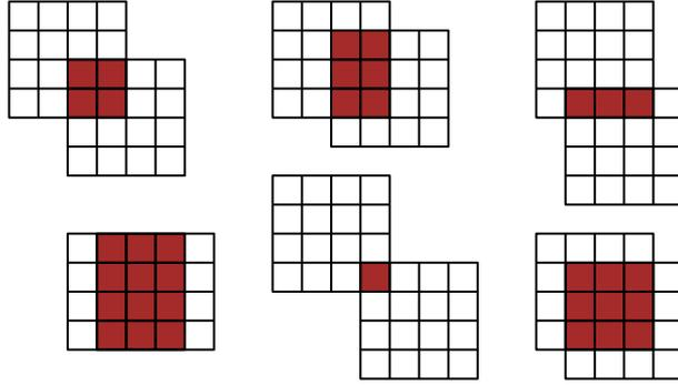
Fig. 3. Different configurations for the support intersection of *two* cubic B-splines. The integrals in (21), corresponding to one look-up operation, are nonzero only for tensor B-splines  $T_{\mathbf{k},q}$  which possess a non-empty intersection with the filled region.
