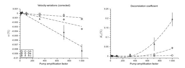
Figure 6 : Pump amplitude dependence of CWI measurements: a) Corrected velocity variation  $\alpha$  vs. normalized pump amplitude and b) Remnant correlation coefficient Kd vs. normalized pump amplitude. Both the linear and quadratic fits are proposed. Standard deviations are indicated.
