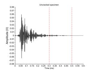
Figure 3 : Temporal coda signals recorded and time-window used for CWI analysis.
