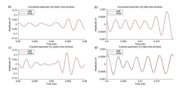
Figure 4 : Temporal coda signals recorded and time-window used for CWI analysis: a), b) an uncracked specimen (A), c) and d) for a cracked specimen (C) with two different pump wave amplitudes Apump (0 dB and 60 dB). a) and c) are close-ups of the coda signals during an early time interval (20-s wide); and b) and d) are close-ups of the coda signals during a late time interval (20-s).
