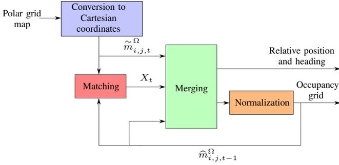
Fig. 1: Overview of the Evidential SLAM algorithm
