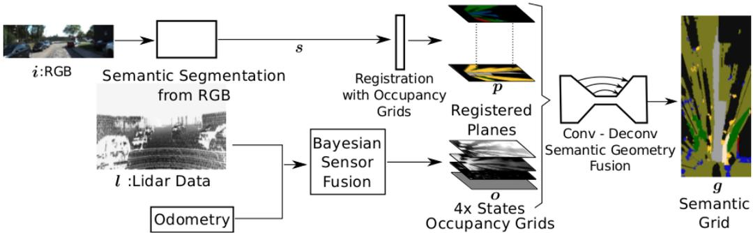
Fig. 2: Functional overview of the method.  $i$ : RGB Image,  $l$ : LIDAR data,  $o$ : occupancy grids,  $s$ : output of the segmentation network,  $p$ : registered planes as inner representations,  $g$ : semantic grid
