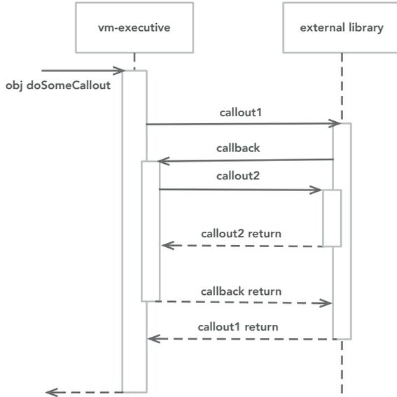
**Figure 3. Reentrant callouts in the presence of callbacks.** Callout2 is a reentrant callout, executed during the dynamic scope of callout1’s execution. This happens because a callback gives back the control to the vm-executive, allowing new callouts before callout1 finishes.
