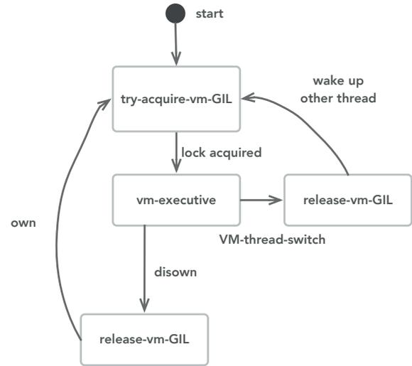
**Figure 2. Illustrated life-cycle of a VM thread in the presence of VM thread-switch.** When a green thread *affined* to a VM thread different than the current one is scheduled to run, the current VM thread releases the GIL and the *affined* VM thread is awoken.
