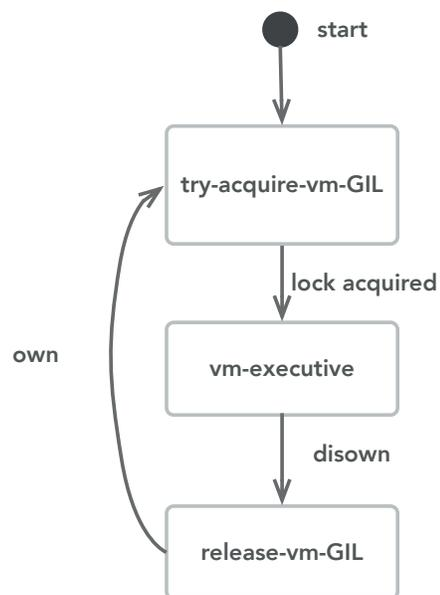
**Figure 1. Illustrated life-cycle of a VM thread in the presence of I/O.** The GIL is acquired before entering the vm-executive, and released on I/O operations. When the I/O operation finishes the VM thread attempts to re-acquire the GIL.
