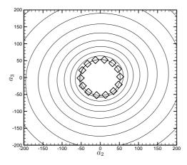
Fig. 11. Comparison of the projected (NS:  $\Diamond$ ) and the predicted (ROM: ——) limit cycles over 1000 vortex shedding periods. 3 modes model.
