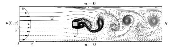
Fig. 1. Flow configuration and vorticity snapshot at Re = 200.
