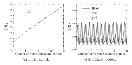
Fig. 18. Temporal evolution of the  $L^2$  norm of the Navier-Stokes residuals computed using a 3-modes ROM.
