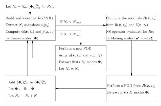
Fig. 20. Schematic representation of the functional adaptation process based on a Krylov-like method.
