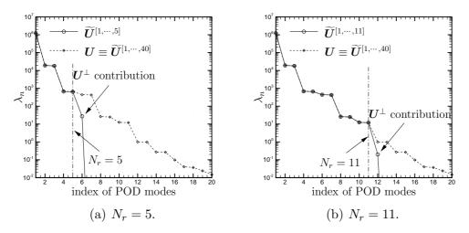
Fig. 25. Comparison of the temporal correlation tensor eigenvalues evaluated from the exact field, U, and from the  $N_r$ -modes approximated one,  $\widetilde{U}^{[1,\dots,N_r]}$ .
