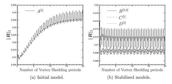
Fig. 17. Temporal evolution of the  $L^2$  norm of the Navier-Stokes residuals computed using a 5-modes ROM.
