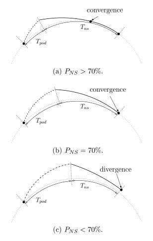
Fig. 28. Schematic explanation for the convergence of the hybrid DNS-POD method. .... exact "target"; -- POD ROM; ——— DNS.
