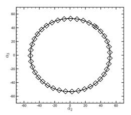
Fig. 16. Comparison of the projected (NS:  $\diamondsuit$ ) and the predicted (ROM: —) limit cycles over 1000 vortex shedding periods. 3 modes model with stabilization. (Indistinguishable difference between models  $B^{[3,2]}$ ,  $C^{[3]}$  and  $D^{[3]}$ .)
