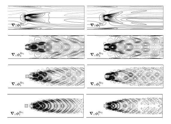
Fig. 19. Comparison of the iso-vorticity representation of some POD modes. The initial POD basis at  $Re_1 = 100$  (left) and the target POD basis at  $Re_2 = 200$  (right). Dashed lines represent negative values.
