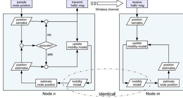
Figure 1: Flow chart of ARH execution. Node  $n$  transmits ‘hello’ message according to the accuracy of its location estimates produced by an AR-based mobility model. Node  $m$  maintains a mobility model for  $n$  that is identical to the one maintained by  $n$  itself.
