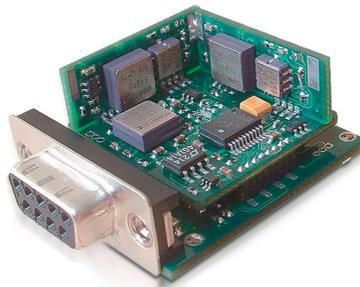
FIGURE 4.8 – Centrale inertielle Crista de Cloud Cap Technology.
