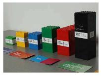
Figure 2: The data-sculpture set of blocks (data sculpture + TUI). Prototype of tangible interface and data sculpture representing six radio stations. The height of the block represents the *number of listeners* and the depth of the block represents *the total time listened*.
