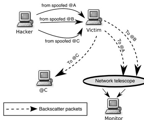
Fig. 1. Backscatter principle
