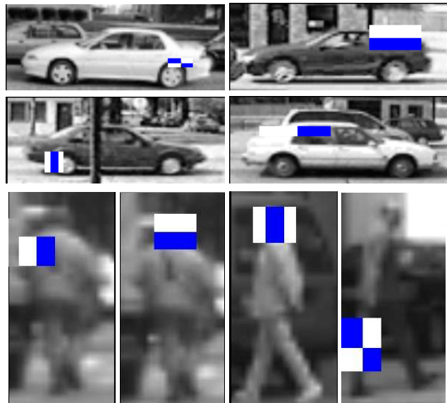
Fig. 2: Some examples of adaBoost-selected Viola-Jones features for car detection (top) and pedestrian detection (bottom).
