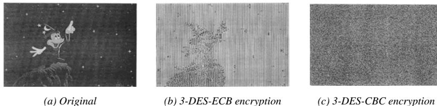
Fig. 1. Encryption opacity.
