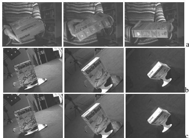
Figure 1. Experiment on the rice box. (a) some of the reference images of the texture models are show, one per face, (b) and (c) results using respectively criterion \Delta_{1b} and \Delta_{1a} . The tracking succeeds when using the best criterion (b), despite permanent specularities. Drift occurs at the end of (c) on the right.
