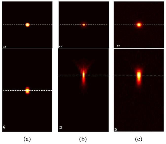
**Fig. 2:** Lateral (top) and axial (bottom) sections of the (a) simulated band-limited microsphere, (b) the theoretically modeled PSF (5) at a depth of  $10\mu\text{m}$ , and the corresponding (c) blurred-noisy simulation of the object as imaged by a CLSM (© Ariana-INRIA/I3S). The intensity is linearly scaled between  $[0, 1]$  for display and the dotted lines shows the sections in the volume.
