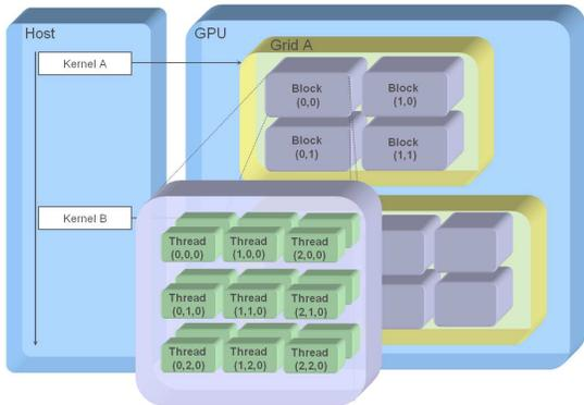
Figure 4: CUDA Programming Model: Grids of Thread Blocks.
