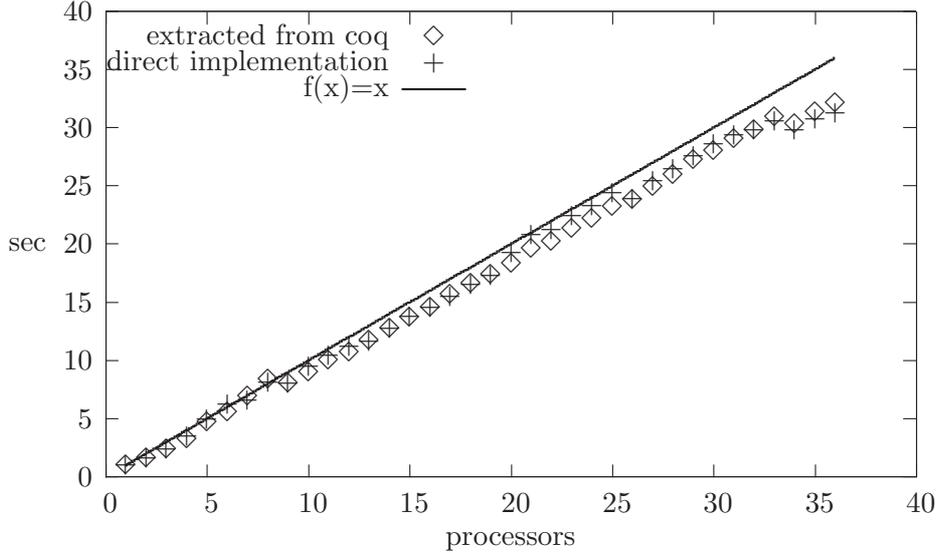
Figure 10: speedup of direct implementation and extracted implementation over 5120000 elements (calculated from computation + GC timings)
