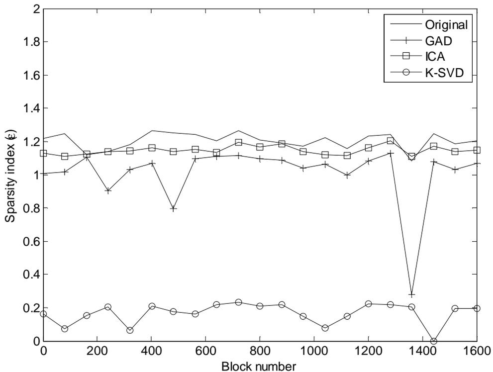
Figure 2 Sparsity index for the GAD algorithm, compared to the original signal, and to ICA and K-SVD for every block in the observation matrix. The GAD algorithm consistently achieves a sparser representation than ICA, but not as sparse as K-SVD.
