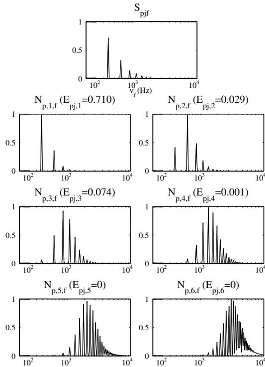
Fig. 2. Basis spectrum  $S_{p,jf}$  estimated for the piano excerpt in Fig. 1 given fixed harmonic fine structure spectra  $N_{p,kf}$  ( $p = 60$ , gammatone windows of order  $n = 4$ ,  $b = 11/3$  ERB,  $K_{\max} = 6$ ).
