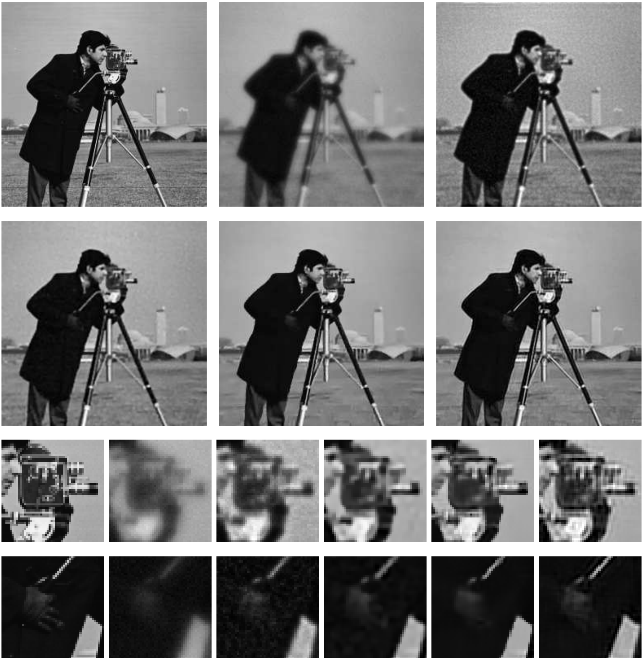
Fig. 2 Examples of deblurring for the case 3. First two line, from top to bottom, left to right: original image, blurry image, Richardson-Lucy, sparse gradient [15], SA-DCT [10], our method. Last two lines: close-ups in the same order. Best seen by zooming on a computer screen.
