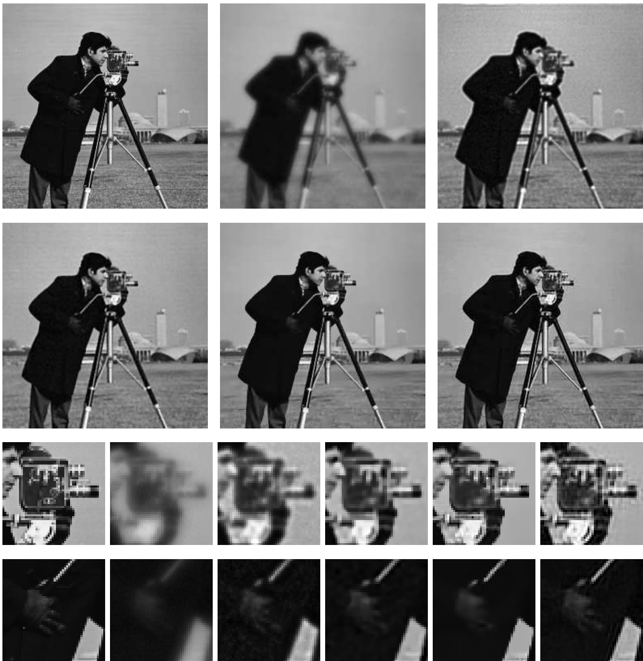
Fig. 1 Examples of deblurring and close-up for the case 2. First two lines, from top to bottom, left to right: original image, blurry image, Richardson-Lucy, sparse gradient [15], SA-DCT [10], our method. Last two lines: close-ups in the same order. Best seen by zooming on a computer screen.
