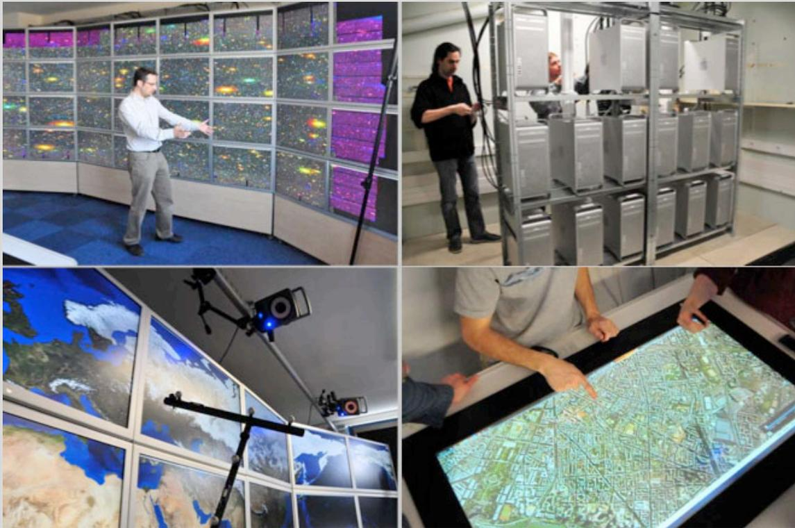
The WILD room (**W**all-size **I**nteraction with **L**arge **D**atasets) features a large wall display (top, left) powered by a 16-computer cluster (top, right) and two front-end computers, a motion tracking system (bottom, left), and an interactive table (bottom, right).
